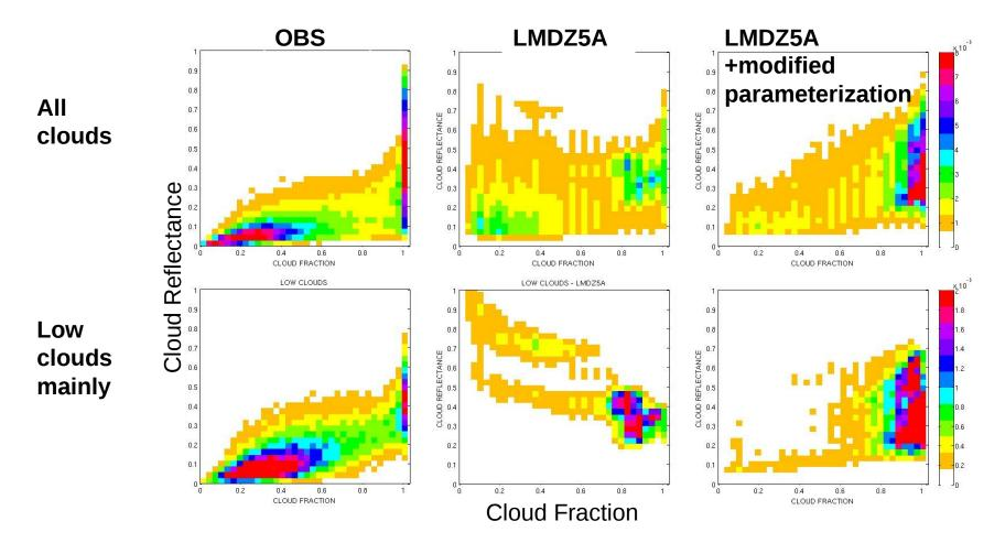
$\rightarrow$  Modified parameterization (considering the horizontal heterogeneity of cloud layers, talk J.L. Dufresne) leads to the cloud reflectance increasing with cloud fraction : consistent with observations
